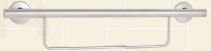
NEWPORT BAR GW-3900 SERIES The one-piece welded construction of this versatile combination grab bar and towel bar offers solid support. Available in a variety of decorative flange options, finishes and sizes. LENGTH: 30" (SHOWN: GW-3930-QCR)
