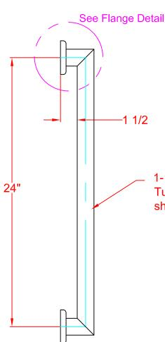
1-1/4" x 18ga. S.S. Round Tubing formed to eliptical shape of 1-1/2" x 1"
